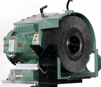
Easily mount a wide variety of wheels up to 3" wide. The side door is a hingeless design with only a single clip for access to the wheel.
