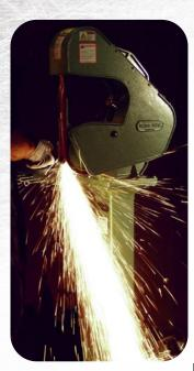
Contact wheel grinding is the most aggressive type of grinding and should be used when heavy stock removal is required. Each elastomer tired aluminum contact wheel is precision machined and balanced for smooth operation. It has been said, when compared to a bench grinder, "that grinding on a Burr King is like grinding on velvet."
