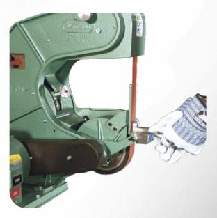
The backup platen provides a large surface area for flat grinding and may be removed when not in use.
