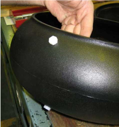
Remove supplied plugs with a 9/16" wrench.
