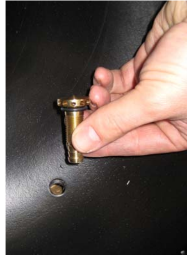
Install drain plug thru the bottom of the bowl making sure that the rubber o-ring is properly seated to the bowl.
