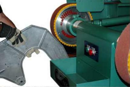
Standard 14" diameter contact wheels available in widths of 2"-3" or 4"
