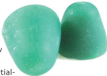
**SYNTHETIC:** A blend of urea formaldehyde resin and abrasive material, such as aluminum oxide or silicon carbide. Synthetics provide environmental benefits due to its clean, non-foaming residue. Synthetics however have a lower specific gravity than plastic, meaning they do not remove material as aggressively. This type of media is a good choice for delicate parts. Synthetics do have a higher wear rate than plastic.
