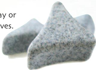
**PLASTIC:** A abrasive which is a petroleum-based plastic media Normally used on non-ferrous materials such as aluminum. Most commonly used when a low RMS micro-finish is desired, or where the finish must be substantially free of impingement damage which is seen if using ceramic media on aluminum or soft material.
