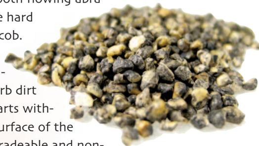
**TREATED COB:** Corn cob treated with aluminum oxide and used for polishing ferrous or non ferrous soft metals. Works well for aluminum.
