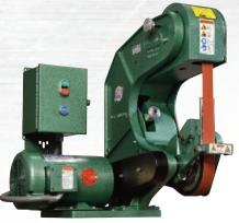
Optional magnetic starters provide safe and efficient 3 phase power
