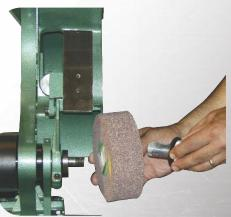
Easily mount surface conditioning wheels up to 2" wide with available wheel adapters.
