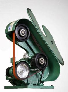
Urethane idler wheels are long lasting and electronically conductive
