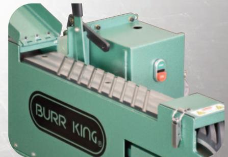
3" x 18" replaceable serrated platen for the jobs that need to be flat.
