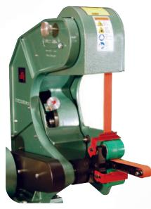
The 1400 series small wheel attachments allow you to grind in places you wouldn't have dreamed of before. Wheels from 9/16" to 1.5" in diameter are available.
