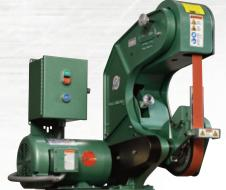
Optional magnetic starters provide safe and efficient 3 phase power
